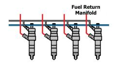
Fuel return manifold carries away fuel that was not injected for combustion
