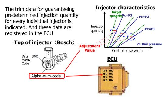
ECU has an injector Trim data for each cylinder. At the time of injector exchange, the trim data in ECU needs to be rewritten using the Yanmar SmartAssist-Direct (SA-D).
